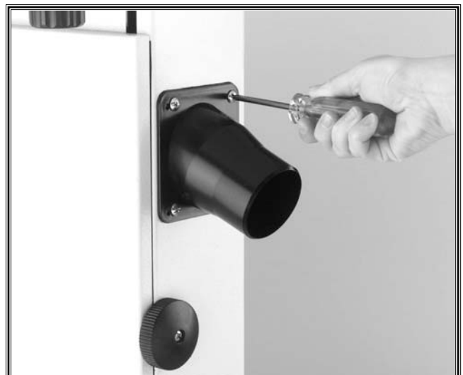
Figure 19. Installing dust port.
